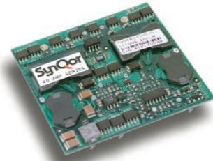
**Figure 4:** SynQor converter with no heatsink or baseplate
