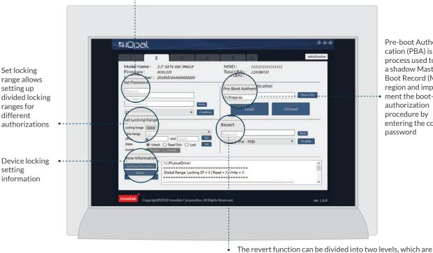
Pre-boot Authentication (PBA) is a process used to add a shadow Master Boot Record (MBR) region and implement the boot-up authorization procedure by entering the correct password
