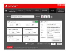
The Alert tab helps the user set trigger points with Temperature, Health Percentage, Remaining Capacity or Life Remaining. If these trigger points exceed their boundaries, the iSMART utility can send a warning and email to the user, notifying them that something is at risk of failing.
