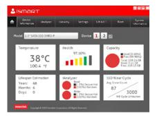
The Dashboard's home provides a quick snapshot of each installed device in the system. This page offers accurate data information regarding Temperature, Health, Capacity, Lifespan, iAnalyzer, and Notifications. Further device information such as S/N, firmware version, interface, etc. is also available.
