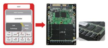
iCell technology gives the SSD a power boost in the event of an abnormal power failure and ensures reliable and accurate data transfer from DRAM cache to NAND flash.
